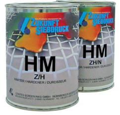
Pot life varies from ink range to ink range. Inks should not be printed after this period of time as then the printed ink film will not exhibit the required resistances due to the progressed cross linkage reaction with the hardener. Following initial drying 2-component inks will require periods of up to 6 days (depending on curing temperatures) to achieve a complete cross
